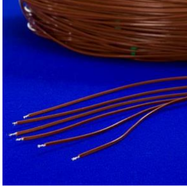
Validation Thermocouple Looms
